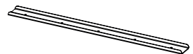
2 x N - 1 x reinforcement profile (if distance between legs is greater than about 2300 mm)
