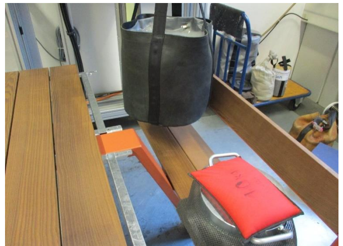
Abb./Pic. 16: Seating durability test
