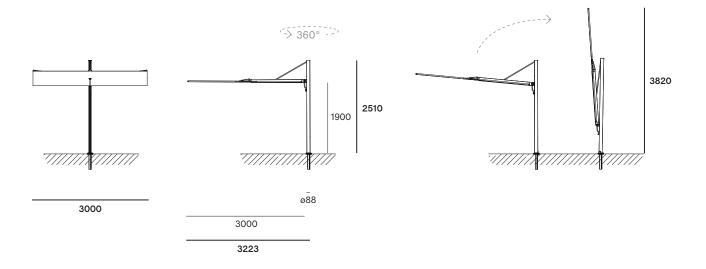
In combination with the permanent fixation & pole extension (360 degree rotatable)
