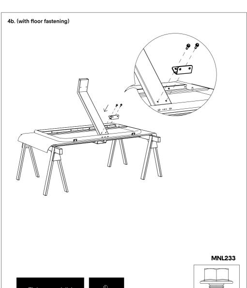
**Tighten carefully!** Excessive force may damage the coating!
