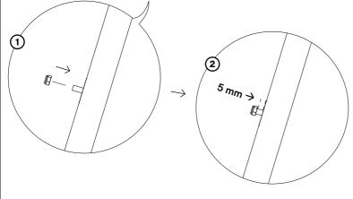
Screw the nuts about 5 mm onto the threads
