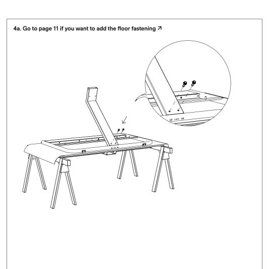
Tighten carefully! Excessive force may damage the coating!
